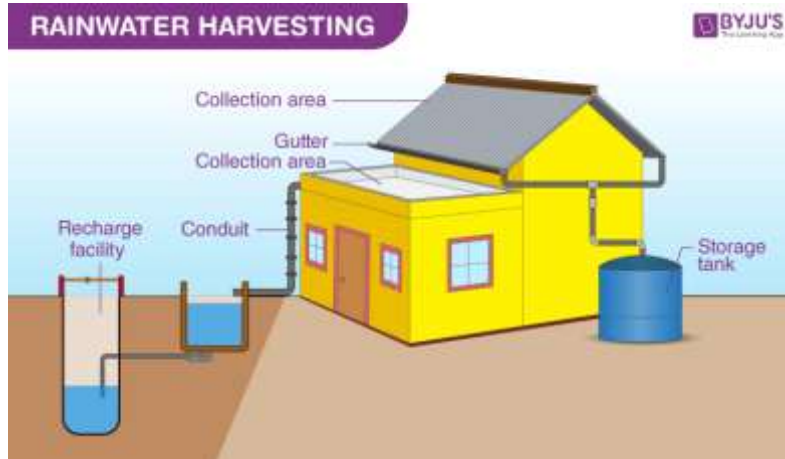
Fig. 1 Rainwater Harvesting System – Concept & Components
