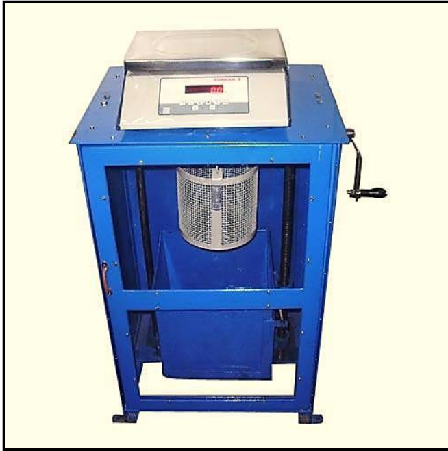
Figure 3 Specific gravity and water absorption are measuring instruments in the laboratory
